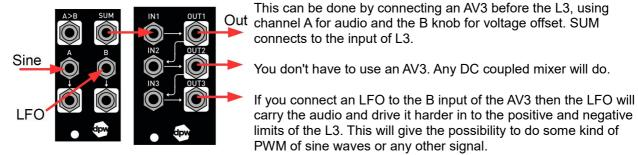
You can as shown in the picture like in the waveshaping example get different versions of this PWM like signal out if you don't connect anything in on channel 2 and 3.
