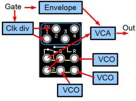
This is a patch making drum sounds with only one VCA, one envelope, a clock divider and 3 sound sources. Two channels of the switch will be used.
