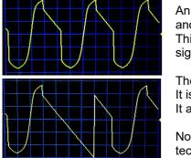
An example of where the PWM signal is switching from the sine to the saw and back. Replacing parts of the sine wave.
