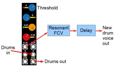
The drums are just passing though the modules B channel here.
