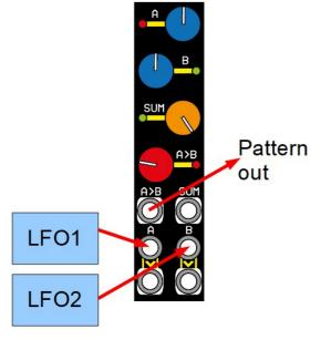
The AV2 can be used to produce pseudo-random like rhythm patterns to trigger other modules. For example drums.
