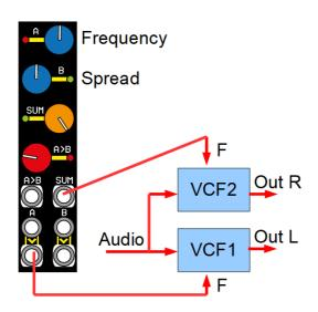
This example shows how to filter a mono sound into stereo.
