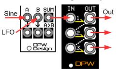
This can be done by connecting an AV-1 before the L-2, using Out channel A for audio and the B knob for voltage offset. SUM connects to the input of L-2.
