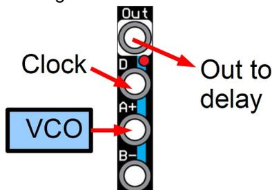
One example is to connect it on the clock input of a delay to get slight frequency shifting on the output.
