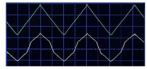
With Mod set from off to middle position the WF-1 can act as a compressor. On the picture you can see how the amplification of the triangle wave decreases after a set value at OffP and OffN.
