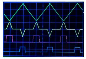
If Clean is set to max anticlockwise (off) the OUT signal will change to be as the yellow signal on the picture.
